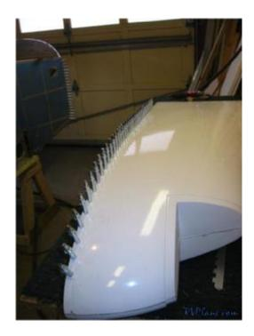
6) Next step is to drill the wingtip-side hinge – the thinner 'P3' hinge. To do this I started off marking where the rivet line should be, using the existing wing-side holes in the wingtip flange as a guide.
