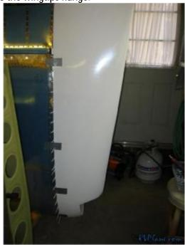
4) The default hole spacing for the #6 screws is too wide for a line of rivets. I used a rivet spanner to drill a new hole in between the existing holes on the outboard edge of the wing skin.
