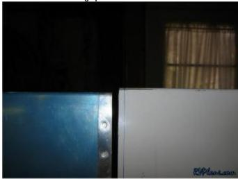
3) Tape the wingtip to the wing using duct tape and use the pre-drilled #40 holes on the outboard end of the wing to drill into the wingtips flange.
