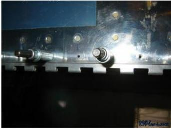
And in this picture, you can see how the flange from the wingtip acts as a spacer between the P4 hinge and the wingtip skin:
