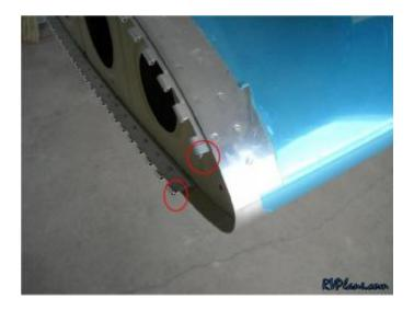
13) The final step is the method to secure the hinge pings to the wingtip rib. I used an old plastic cutting board. I cut it to contour the wingtip rib, and put a #12 hole in the middle of it which is attached to a nutplate.
