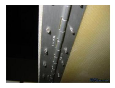
8) With all of the holes drilled in the hinges, it is time to remove the flange from the wingtip. This flange will be used as a spacer on the wing-side so the wing and wingtip are completely flush. I didn't cut the entire flange off – just the portion which had the hinge overlapping with it. I kept the leading edge flange attached to the wingtip.
