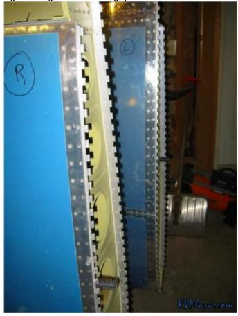
11) For the wingtip P3 hinge to be attached, the wingtip #40 holes need to be countersunk. I used pro-seam to also bond the wingtip hinge to the wingtip, since sometimes rivets can pull out of fiberglass.
