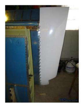
10) Permanently attach the wing side of the hinge to the wing. I dimpled the holes in the skin and countersunk the fiberglass flange from the wingtip.
