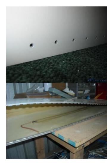
12) In order to only allow the wingtip hinge pins to go so far into the wing, I installed #4 stainless steel screws in the eyelets of the wing-side hinges,
