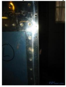
5) The next step is to drill the wider "P4" hinge into the wingtip using the existing holes:
