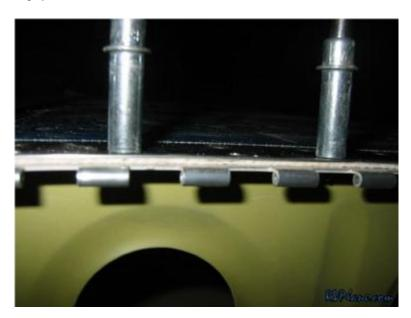
And the test fit. If the hinge pins don't easily go through the eyelets of the hinge, there are a few tricks:
