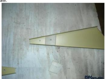
I drilled two #40 holes in the plastic block for the hinge pins to enter. Here is the finished product:
