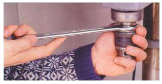
There are two ways to remove most chucks. For chucks without a collar (above), lower and lock the quill and insert an open-end wrench above the chuck. Snap the wrench upward to pop the chuck off. To remove chucks with threaded collars (right), grip a chuck hole by inserting the handle of the chuck-key, and turn the collar clockwise with a spanner.
